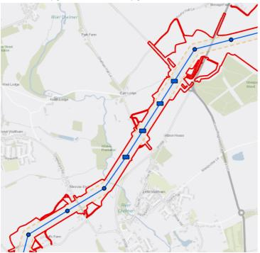
The ES Figure 4.1: Proposed Project Design (document reference 6.4.F1) and Figure 4.2: Proposed Project Design – Permanent Features (document reference 6.4.F2) show pylons TB140, TB141 and TB142 to the south of the River Chelmer as low height pylons.
