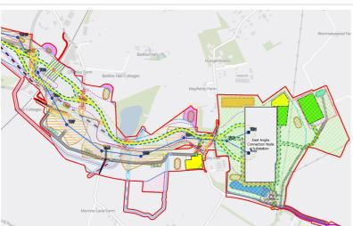
ES Figure 4.1: Proposed Project Design (document reference 6.4.F1) and Figure 4.2: Proposed Project Design – Permanent Features (document reference 6.4.F2) shows an overhead line alignment and underground cable alignment between TB1 and TB8.
