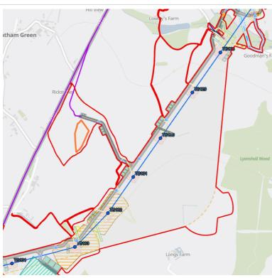
ES Figure 4.1: Proposed Project Design (document reference 6.4.F1) and Figure 4.2: Proposed Project Design – Permanent Features (document reference 6.4.F2) shows an overhead line alignment between TB128 and TB133.
